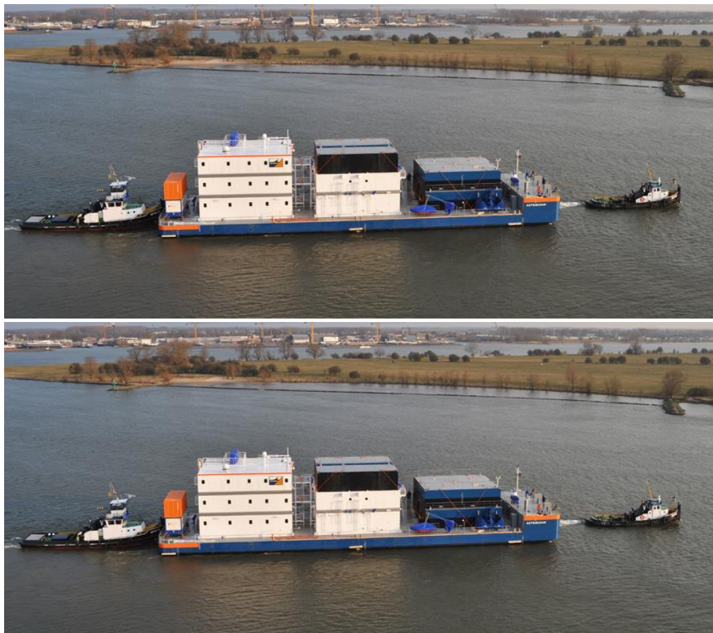
Figure 3: HAR containers placed on a barge
