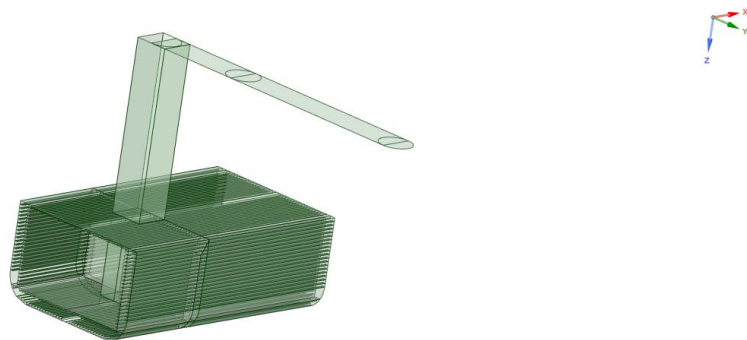
Figure 24: The part of the ship, which was modelled with a rigid crane structure
