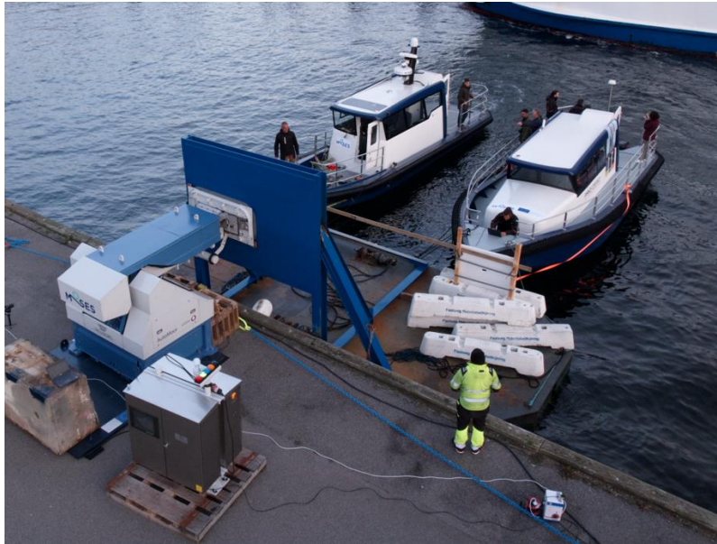
Figure 15: Pilot 1 demonstration, the autonomous tugboats pushing a barge to the AMS.
