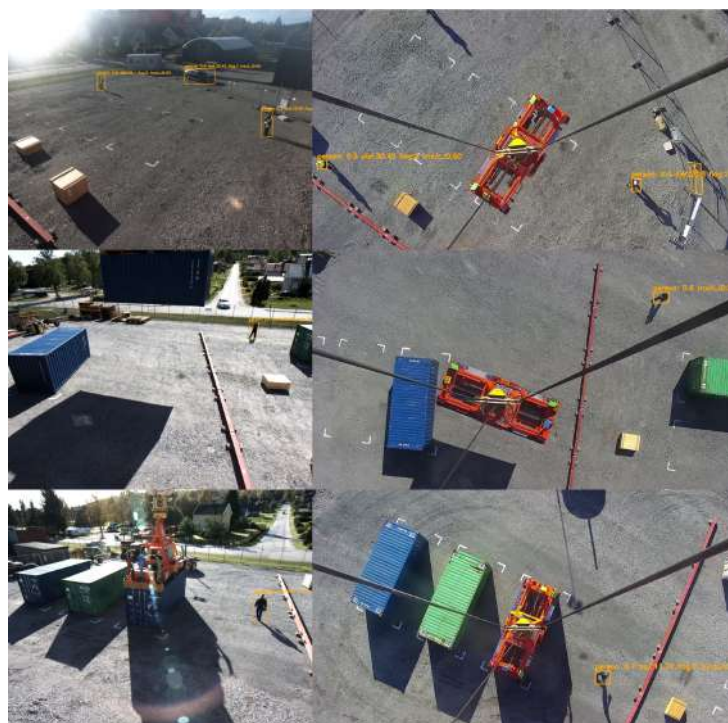
Figure 10. Experiment 6 results. Each row illustrates a scenario in the pilot demonstration. The results of the human activity detector on the oblique image (left) and overhead image (right) are shown. In this test, the emergency stop functionality was disabled, meaning that detected persons are indicated as threats and shown as orange bounding boxes instead.
