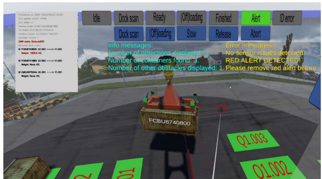
Figure 6. Snapshot of the 3D-Twin for an operational environment with actual containers, showing the spreader with its container, a detected person, the camera's FOV in dark gray, the current work order on the light gray panel, and the system states at the top of the image and blue buttons below for the human interaction.
