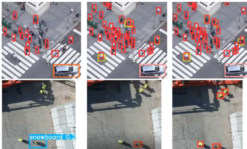
Figure 7. Progressively more accurate detection results for oblique ( top row ) and overhead view ( bottom row ) images that are out of the training distribution. More red bounding boxes means that more persons are correctly detected. From left to right, the results of COCO pretrained, VisDrone trained, and our trained detector.
