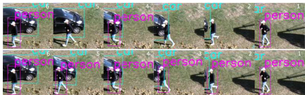
Figure 9. Experiment 5 results. Examples of six consecutive frames (from right to left) of the rooftop dataset without the tracker ( top ) and with the tracker ( bottom ) enabled. With the tracker a person (pink bounding boxes) is detected and tracked more consistently.
