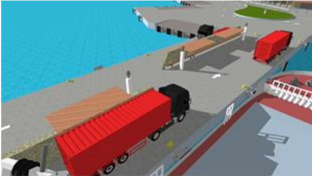
Figure 8. An indication how the situational view could look like. It is a real-time digital twin rendered by IOSS to enable an operator to view an autonomous ship's current situation through virtual reality.
