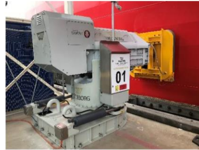
Figure 4: Trelleborg AutoMoor system for automated mooring (left) and a conceptual adaptation for small vessels (right).
